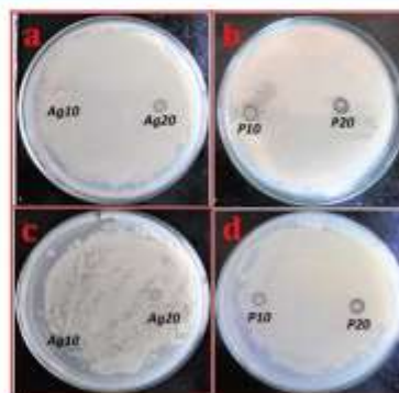
Figure 10. Zones of inhibition of bacteria at 10 and 20 μL/mL of (a) Ag NPs of S. aureus , (b) PANI NFs of S. aureus , (c) Ag NPs of E. coli , and (d) PANI NFs of E. coli .
