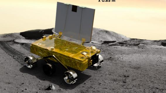
Chandrayaan 2's rover is a 6-wheeled robotic vehicle named Pragyan, which translates to 'wisdom' in Sanskrit. It can travel up to 500 m (0.5 km) at a speed of 1 centimetre per second, and leverages solar energy for its functioning. It can communicate with the lander.
