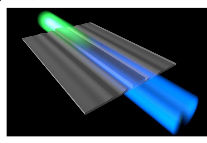
Cooling sound waves with light involves converting sound energy into light energy, which changes the color of the light. (Image credit: Eric Kittlaus and Nils Otterstrom)
