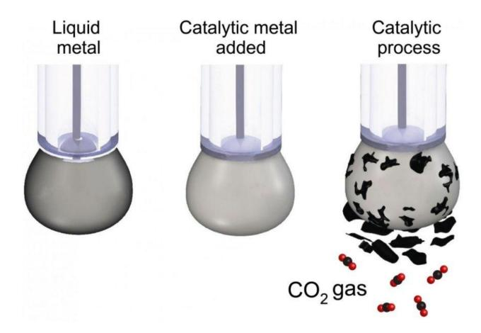
The research team led by RMIT University in Melbourne, Australia, have developed a new technique that can efficiently convert CO<sub>2</sub> from a gas into solid particles of carbon.
